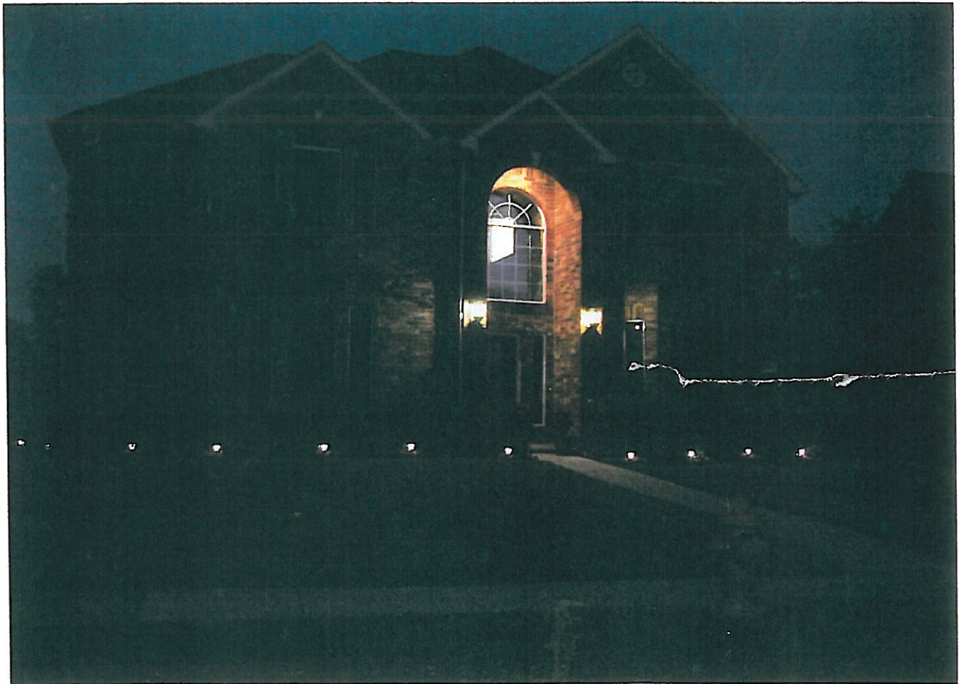
Unacceptable style of low voltage lights that show the light source.
